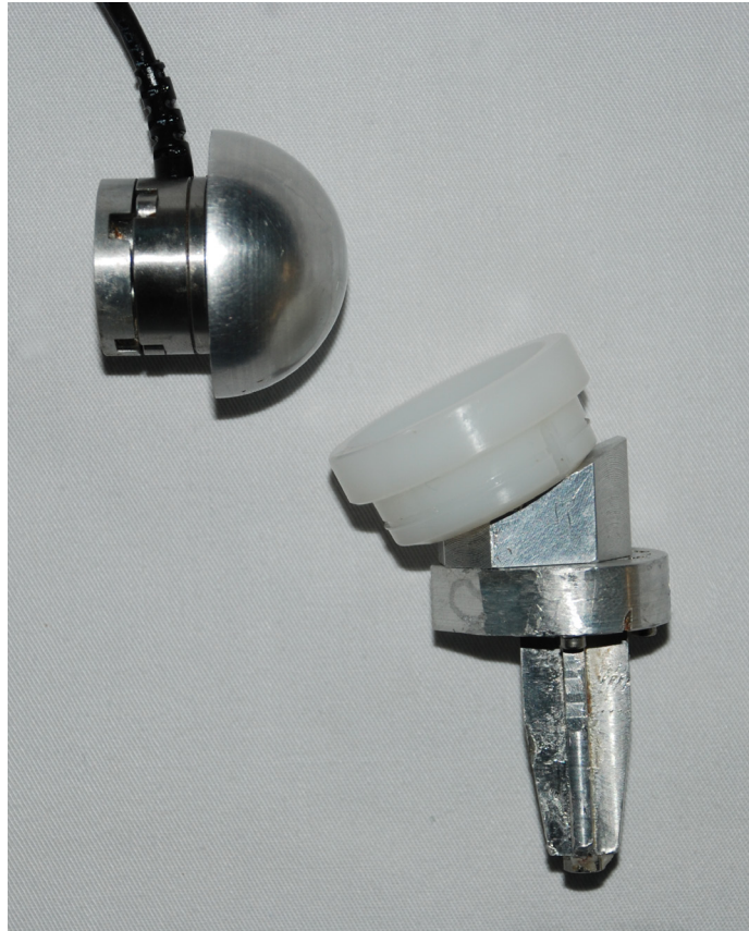
Figure 6.1: Custom modular Reverse Total Shoulder Arthroplasty implants. Photograph showing the humeral and scapular components including the six degree of freedom load cell interposed between the glenosphere and baseplate.
